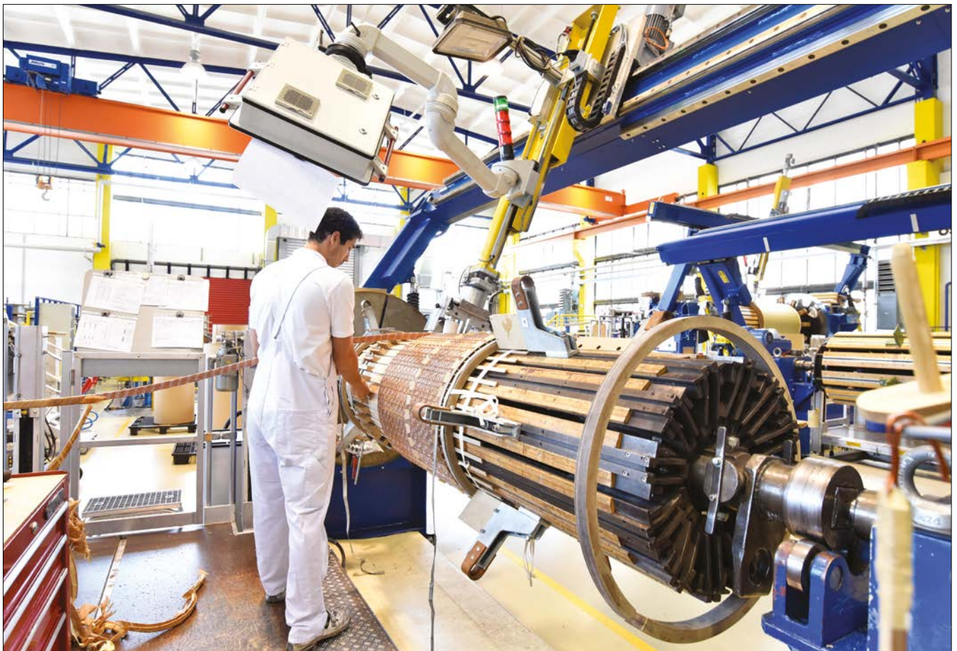
Figure 3. Manufacture of transformers – winding copper wire
