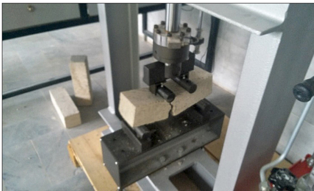
Figure 10: A broken prismatic sample in a flexural test.
