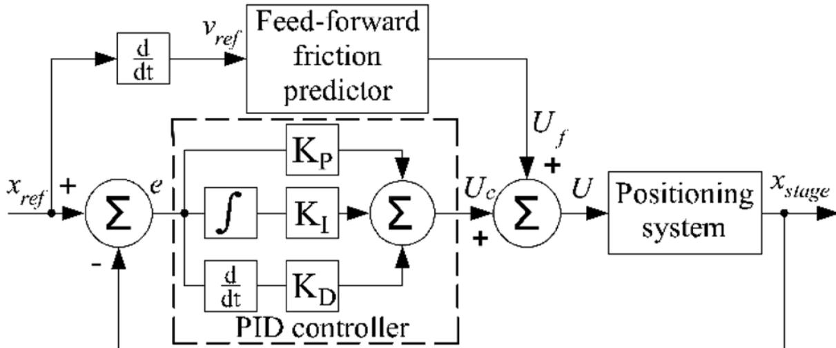
Fig. 3. The control algorithm based on feed-forward compensation of frictional disturbances and a PID
