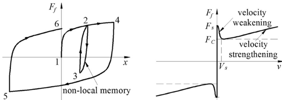
Fig. 1. Friction in the pre-sliding (left) and in the sliding (right) motion regimes
