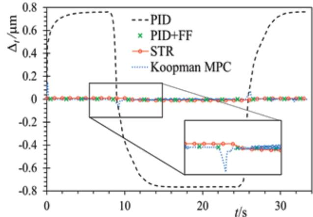
Fig. 9. Tracking errors for different control approaches
