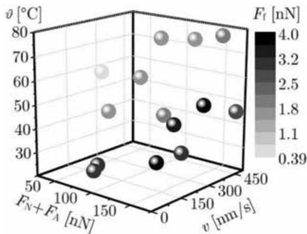
**Fig. 5.** Colour-coded distribution of experimental  $F_t$  values for the test dataset of 15 MC-based points for  $\text{Al}_2\text{O}_3$  [15]
