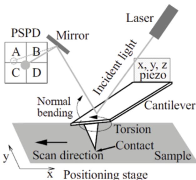
Fig. 2. Scheme of the LFM measurement configuration [6]
