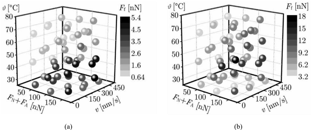
**Fig. 3.** Colour-coded distributions of experimental  $F_f$  values for the 50 CVT DoE points for the  $\text{Al}_2\text{O}_3$  (a), and  $\text{MoS}_2$  (b) samples with adhesion-corrected total load  $F_N + F_A$  [6]
