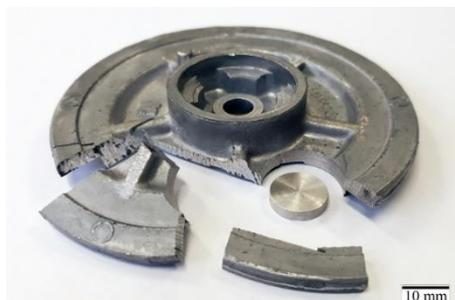
Figure 1. Preparation of samples for microstructural and electrochemical investigations from the automotive parts.
