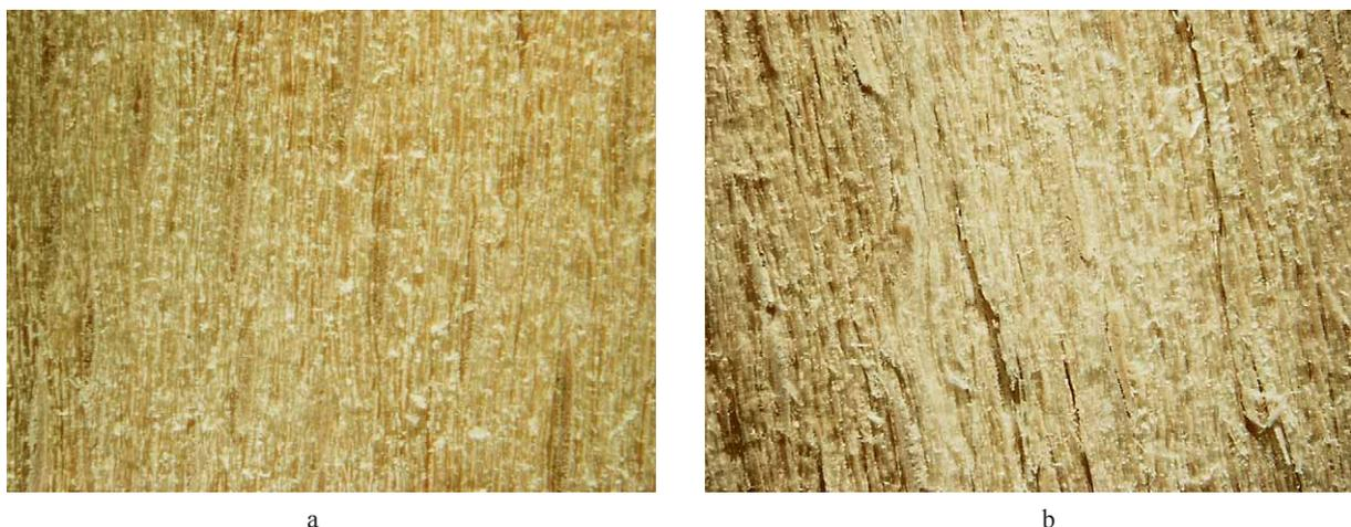
**Figure 3** Micrographs of tight side (a) and loose side (b) of tested veneers – magnification 20x
