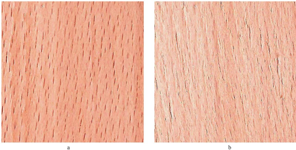
**Figure 2** Macrographs of tight side (a) and loose side (b) of tested veneers - magnification 4x
