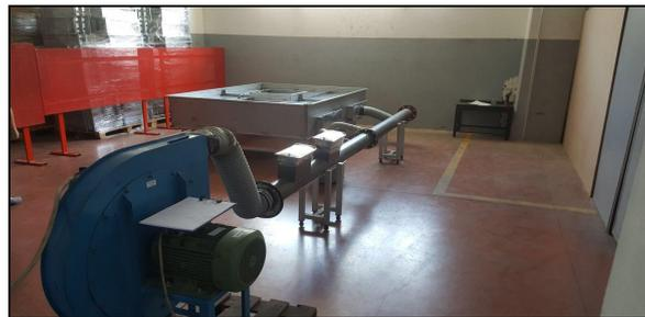
**Fig. 6** Laminar flow tightness test
