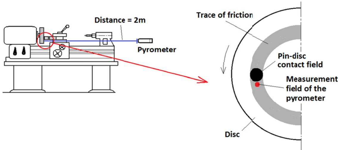
Fig. 2 Diagram of the test bench
