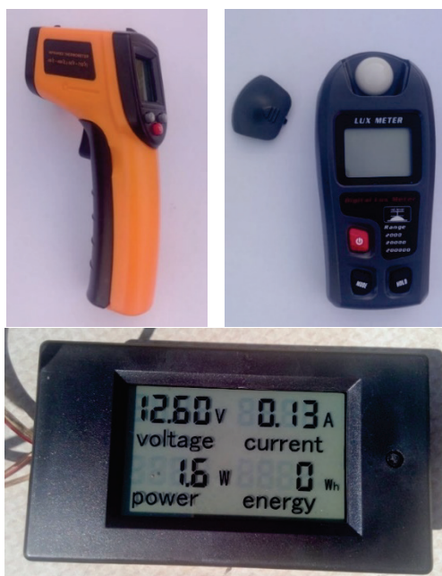
Figure 7 Lux meter Vktech mt30, Thermometer OUTEST GM320 and measuring Module Inpelanyu C01413
