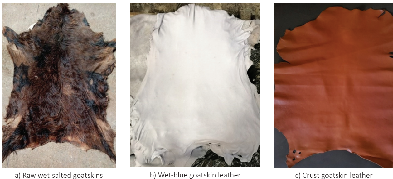
Figure 5. Enzymatically processed goatskin from the raw stage (a), through wet-blue (b) to crust stage (c)
