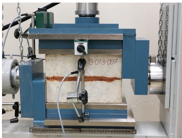
Figure 3: Shear strength test of the built-in filling
