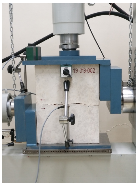
Figure 6: Shear strength test of discontinuities
