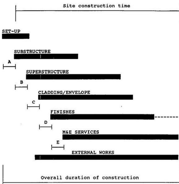
Fig. 1: Simplified outline of the construction plan based on condensed work packages. Source: Nkado (1992).
