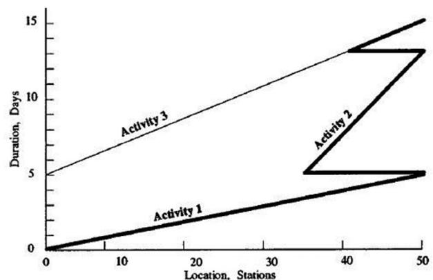
Fig. 2: Example of controlling activity path (CAP) in time–location diagram. Source: Mattila and Park (2003).
