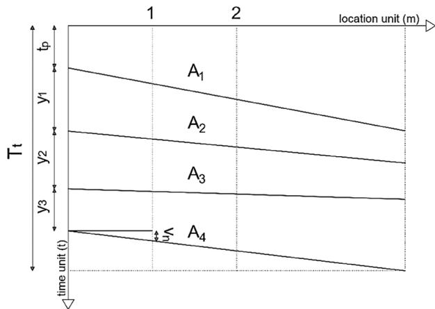
Fig. 3: Graphical representation of the equation of total project time in LSM for continuous full-span activities.
