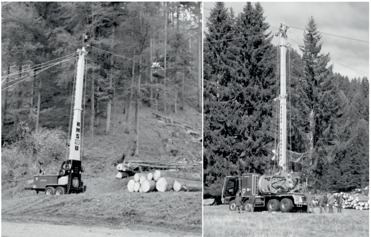
Fig. 3 Left: KMS 12U radio-controlled cable crane ( http://www.excavators-uk.com/konrad.html ). Right: Valentini V1500 tower yarder ( https://www.valentini-teleferiche.it/en/soluzioni/special-machines )
