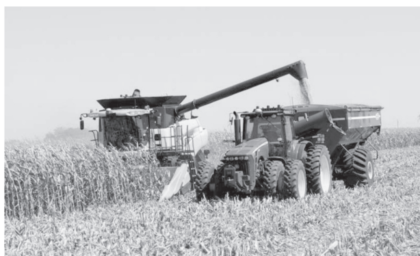
Fig. 7 Autonomous carts (tractor-pulled trailers) – they move between a geo-spatially fixed unloading area and GPS tracker on the harvester (Source: http://robohub.org )
