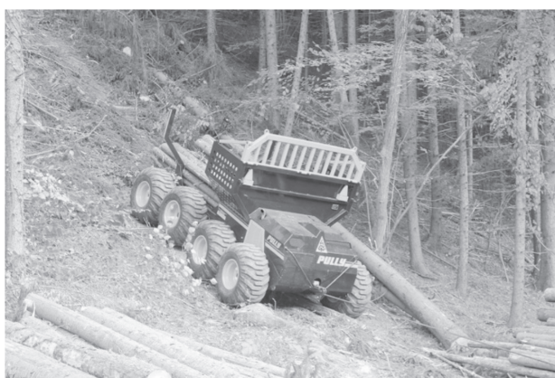
Fig. 8 Konrad »Pully« – takes logs from a steep terrain harvester down to the roadside (Source: https://www.forsttechnik.at/en/products/ground-carriage-pully.html )
