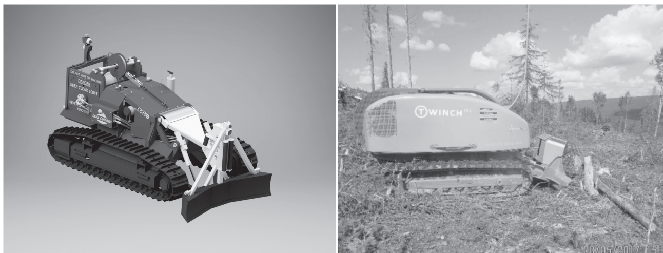
Fig. 5 Remotely operated cabless T-Mar LogChamp 150 (left) and T-Winch (right) winch-assist machines (Photos: T-Mar Industries Ltd. and J. Hunt)
