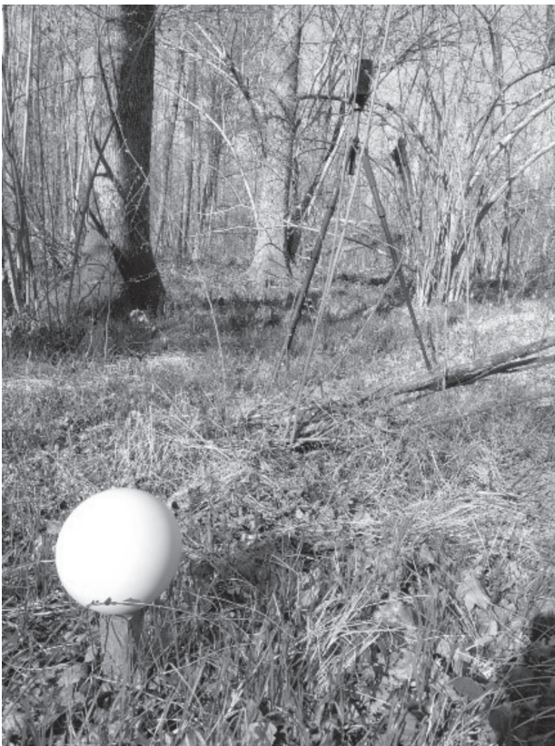
Fig. 3 Sphere placed in forest inventory plot to georeference TLS point cloud
