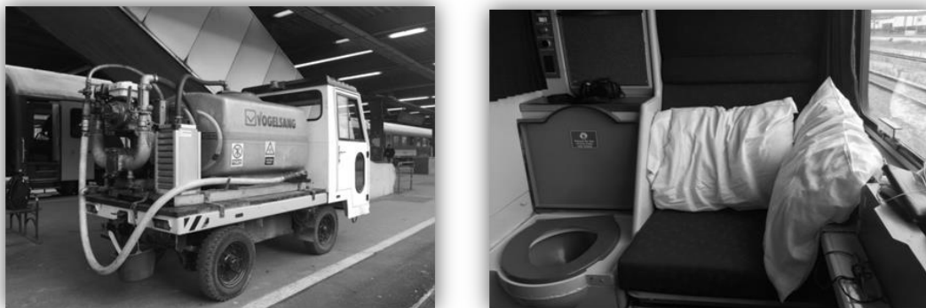
Figure 5. US train toilet at Amtrak/The emptying of closed train toilets at a station.
