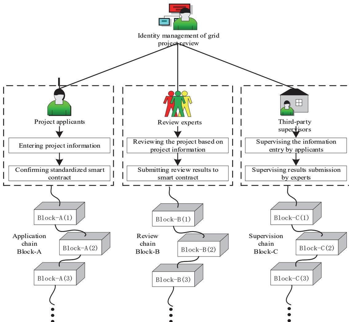
Figure 2 The blockchain-based identity management model for grid project review
