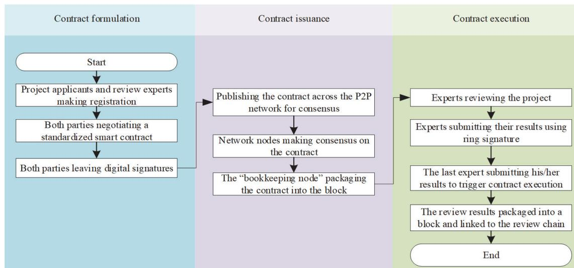
Figure 3 The workflow of grid project review based on smart contract
