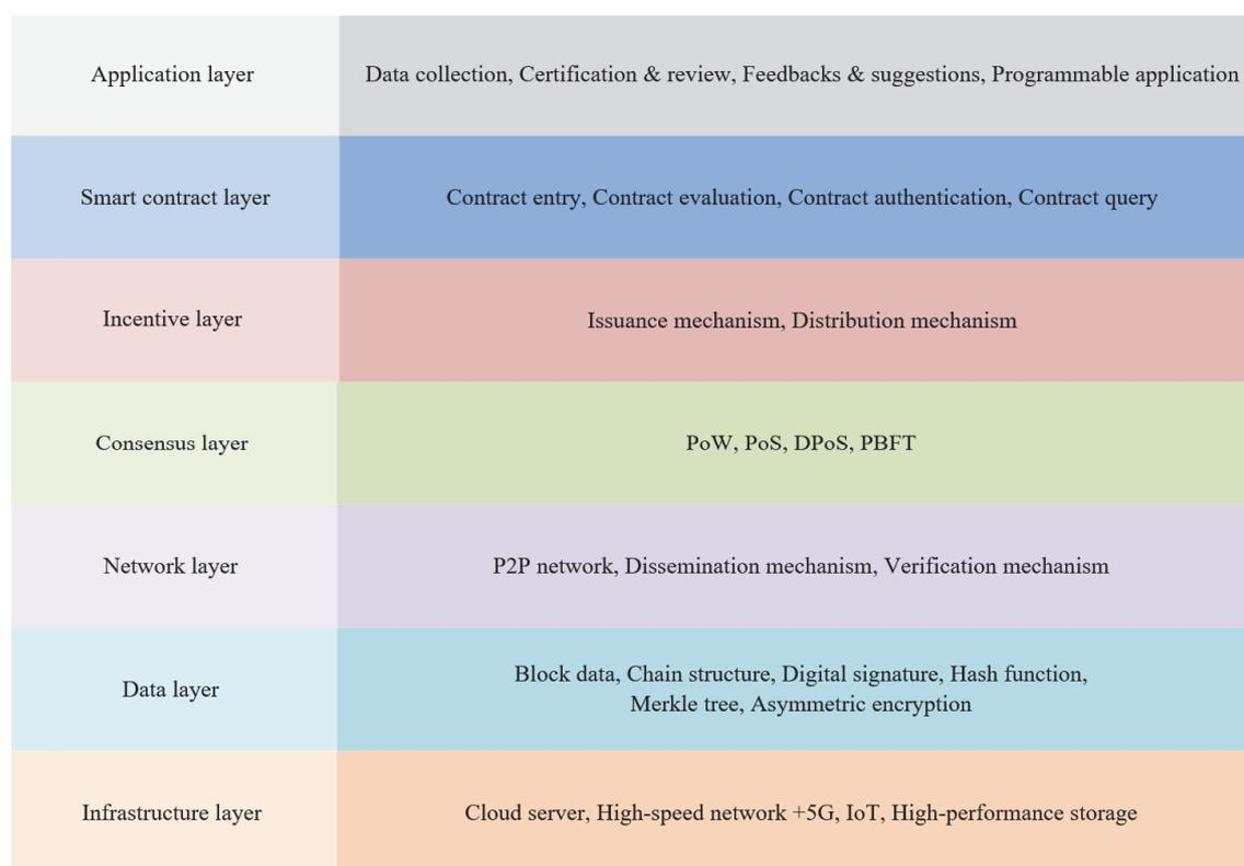
**Figure 1** The architecture of grid project review based on smart contract
