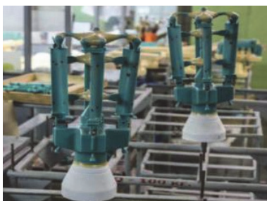
Figure 1 Lost wax method for precision casting of engine blades
