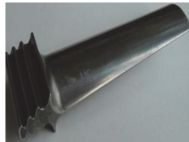
Figure 2 Finished engine blade finished by precision forging
