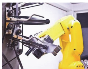
Figure 5 AV&R Aerospace's engine blade polishing system
