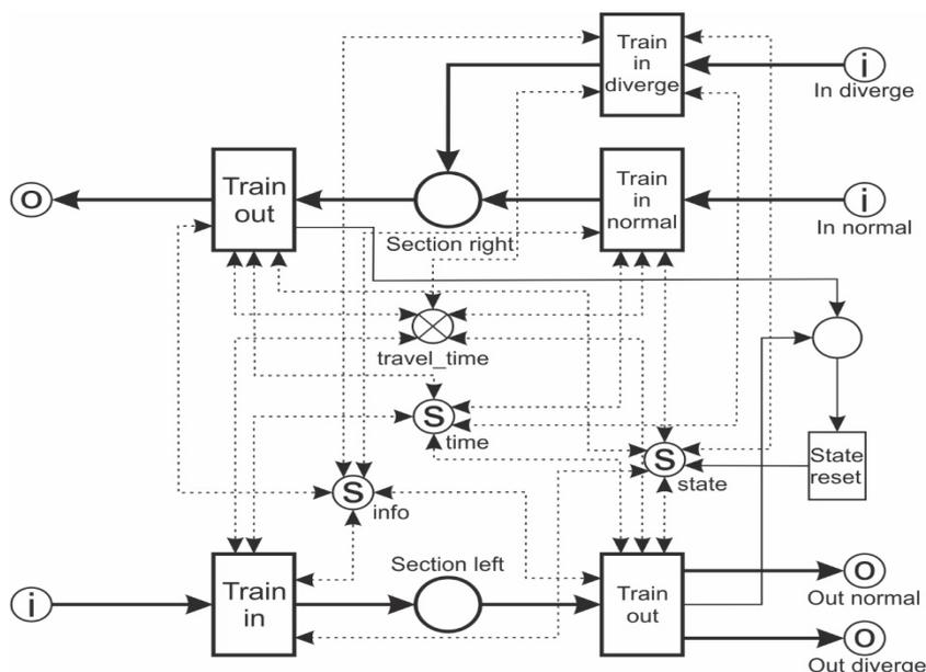
Figure 1 Simple switch module
