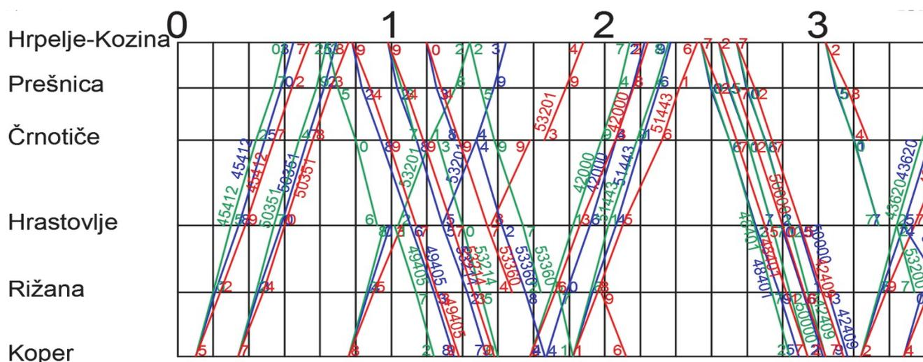
Figure 5 Part of the train graph of Hrpelje-Kozina-Koper railway line from 0:00 - 3:30
