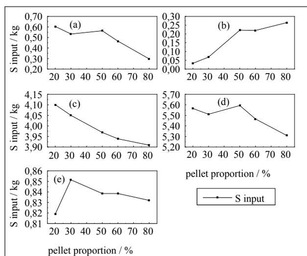
**Figure 3** Sulfur input changes with different pellet proportions in (a) sinter, (b) pellet, (c) coke, (d) pulverized coal, and (e) all raw materials.
