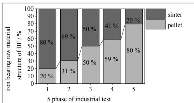
Figure 1 Sinter and pellet proportions in each phase.
