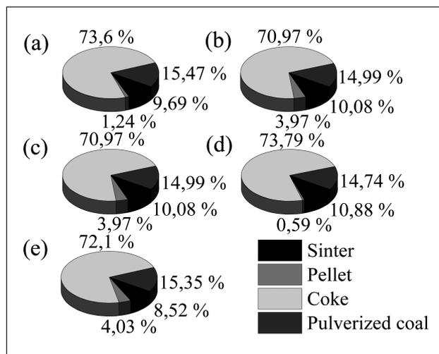
Figure 2 The proportions of sulfur input in each type of raw material with different pellet proportions of (a) 20 %, (b) 30 %, (c) 50 %, (d) 60 %, and (e) 80 %.
