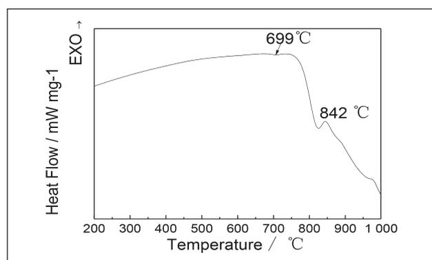
Figure 1 The DSC curves of basic glass
