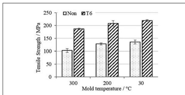
**Figure 9** Tensile strength as a function of mold temperature and heat treatment
