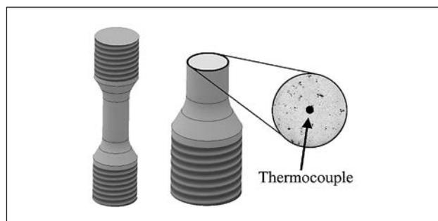
Figure 4 Scheme of sample cooling rate measurement
