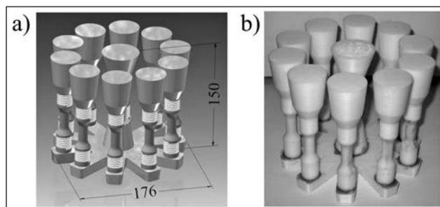
Figure 2 Set of strength samples: a) CAD model, b) printed models
