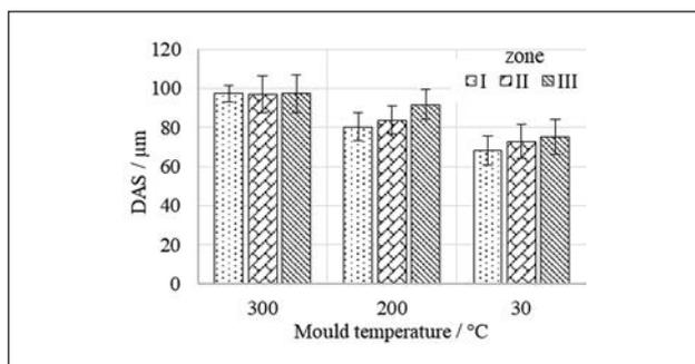
**Figure 8** (DAS) parameter as a function of mold temperature and measurement zone
