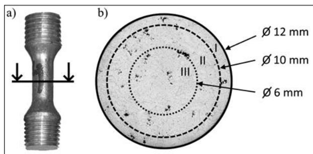
Figure 5 Diagram of the measurement of the (DAS) microstructure parameter: a) place of cutting sample, b) measurement zones
