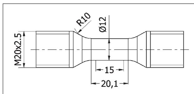
Figure 6 Sample dimensions for tensile strength testing
