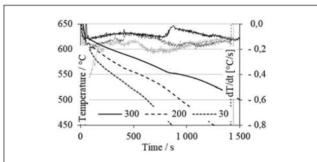
**Figure 7** Cast cooling curves depending on the temperature of the casting mold
