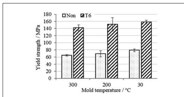
**Figure 10** The yield strength as a function of mold temperature and heat treatment
