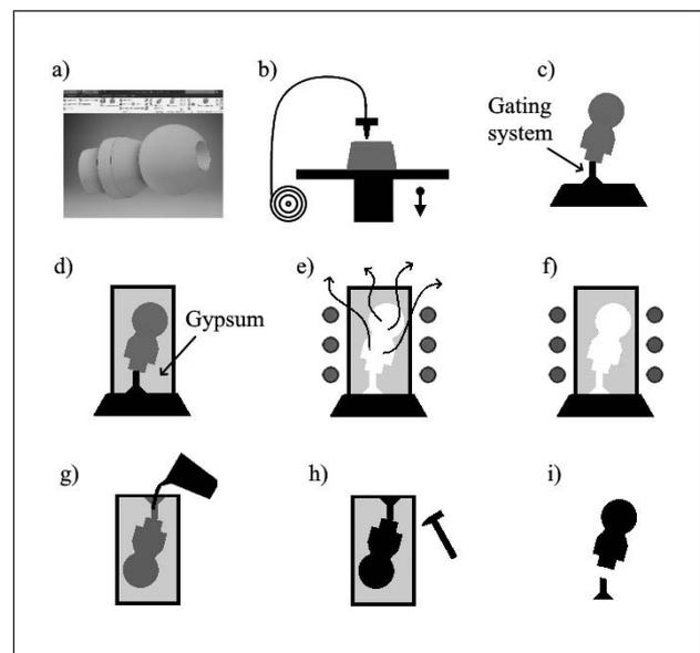
**Figure 1** Gypsum mold process: a) Computer Aided Design (CAD) model, b) Fused Deposition Modeling (FDM) printing, c) insert gating system, d) gypsum mold making e) degassing model, f) mold annealing, g) mold pouring, h) mold destruction, i) cutting and finishing casting
