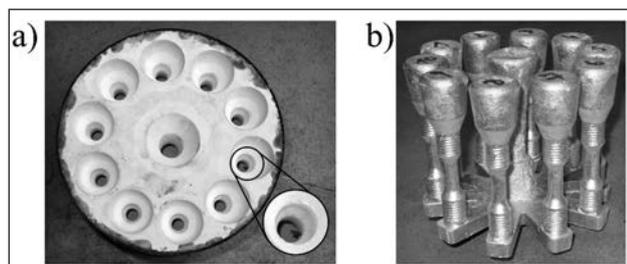
Figure 3 a) Casting gypsum mold with thermo-couple, b) cast strength specimens
