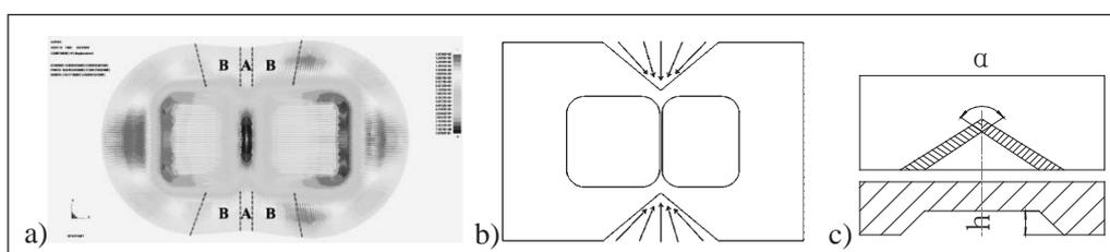
**Figure 5** Material distribution and flow. (a) Material distribution (b) Groove for guiding material flow (c) Structure of guiding groove
