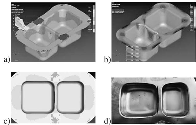
**Figure 4** Simulation and experimental results. (a) Forming limit diagram (b) Thinning rate of material (c) Fracture state (d) Experimental product
