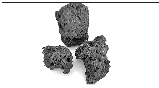
Figure 4 Agglomerate obtained from chromium-nickel ore and semi-coke chromium-nickel ore and Altai's coke
