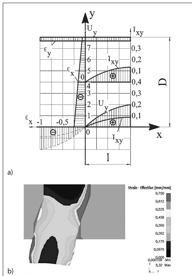
**Figure 2** Deformation state when pulling the workpiece in a special die: a) displacement and deformation fields in the deformation zone; b) deformation values obtained by computer simulation
