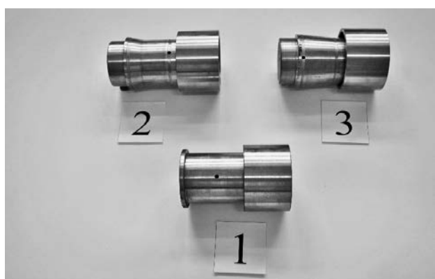
Figure 5 Geometrical shape of the cast iron bushing inner surface: 1 - cylindrical bushing (standard); 2 - bushing with a partial conical bore of the inner cylindrical surface by 0,35 of its length; 3 - bushing with partial tapered bore of the inner cylindrical surface by 0,7 of its length
