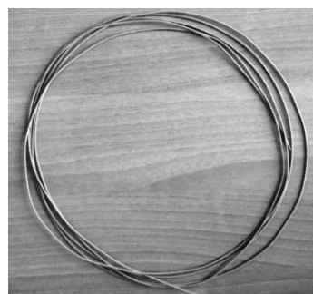
Figure 1 Catamold 316L filament
