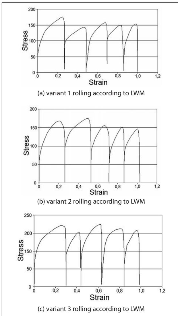
**Figure 3** Change in resistance to deformation at temperature 1 000 °C
