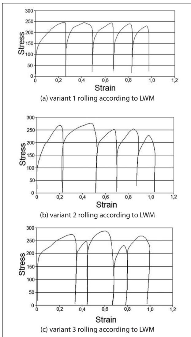
**Figure 1** Change in resistance to deformation at temperature 800 °C
