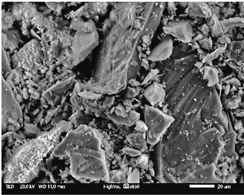
Figure 3 SEM image of Si-based composite powder
