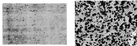
a) Formation a film from silicon powder material by laser printing b) Structure after printing with an optical microscope
