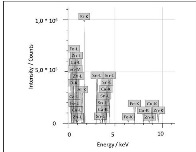
Figure 5 Energy Dispersive Analysis of Silicon Powder
