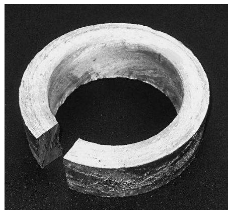
Figure 1 Composite centrifugal casting
