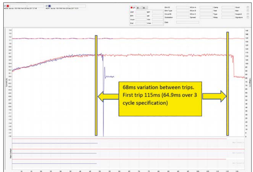
Figure 4. Breaker slow opening time difference
