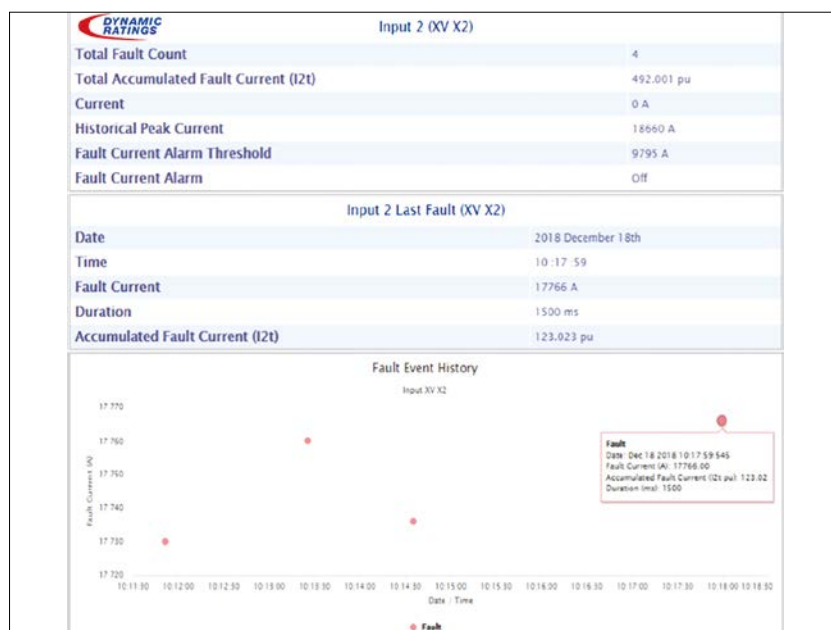
Figure 2. Example of fault counting on the transformer monitor
