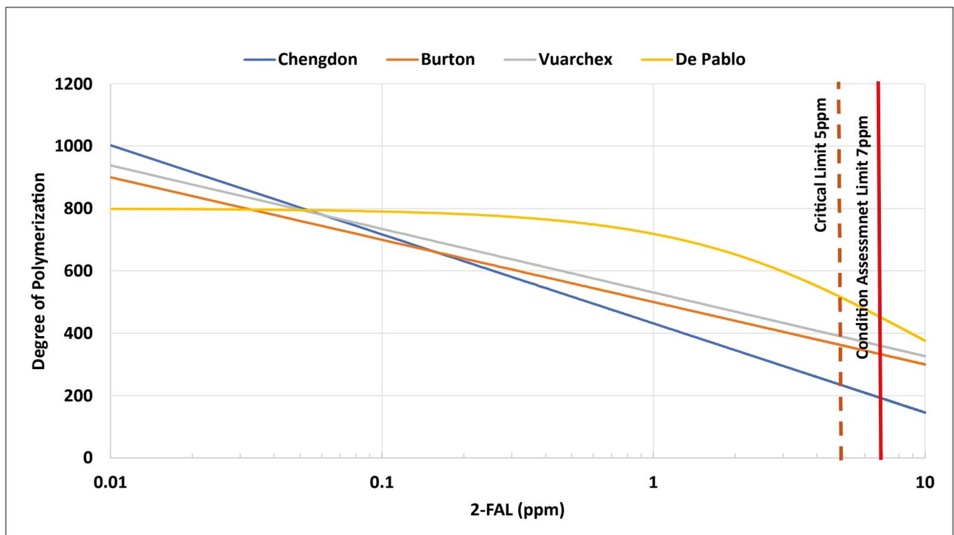
Figure 2. Critical and condition assessment limits based on different DP models [9]
