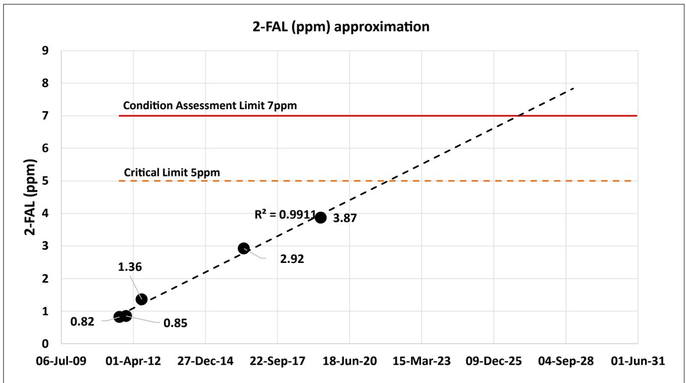
Figure 1. Straight-line trending of 2-FAL over time to estimate transformer retirement age
