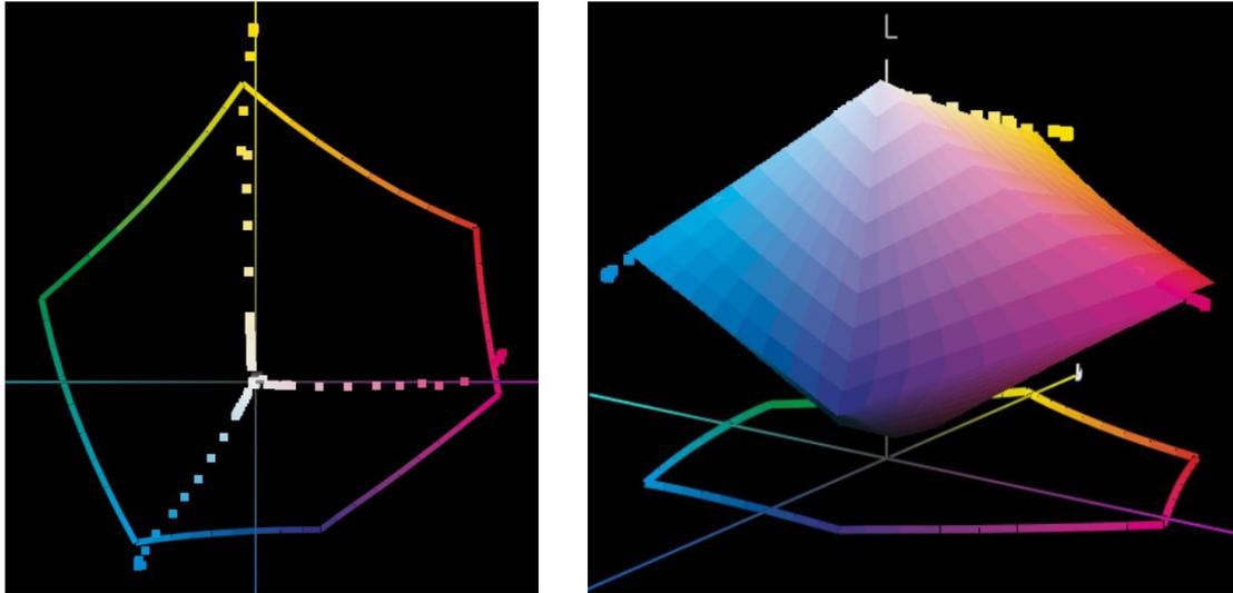
Fig. 5: 2D Plot (l) and 3D Plot (r) of Optimization Run (CMYK) Vs. CRPC 6 GRACoL 2013 Profile
