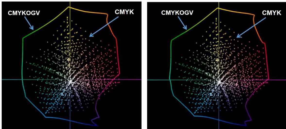
**Fig. 7: Gamut Comparison between CMYK and CMYKOGV with 728 patches (left) and 2016 patches (right)**
