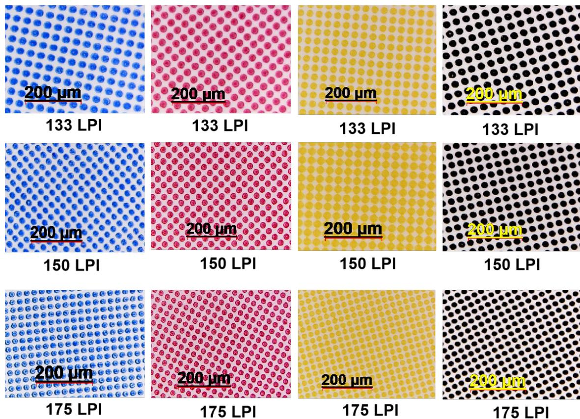
Fig. 3: Dot structure for CMYK at varying plate resolutions
