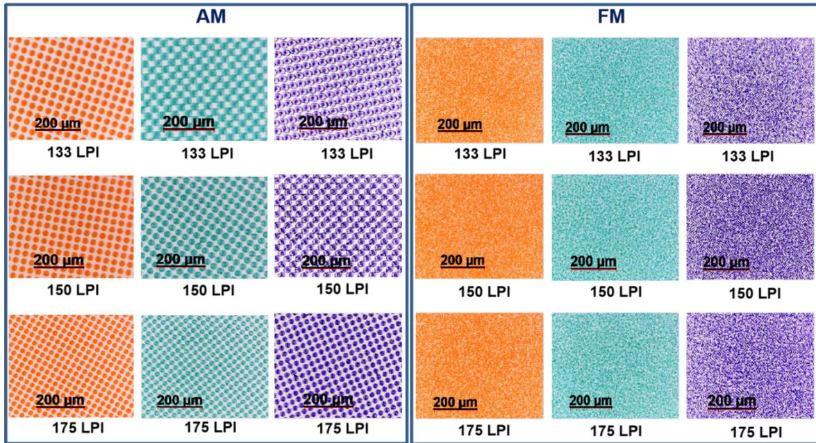
Fig. 4: Dot structure for OGV at varying plate resolution of AM and FM
