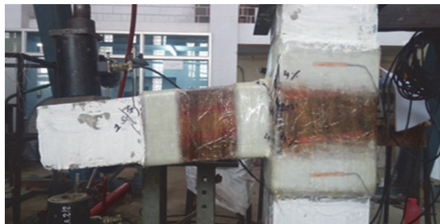
Figure 17. Crack pattern of S2ARF at 5 % drift
