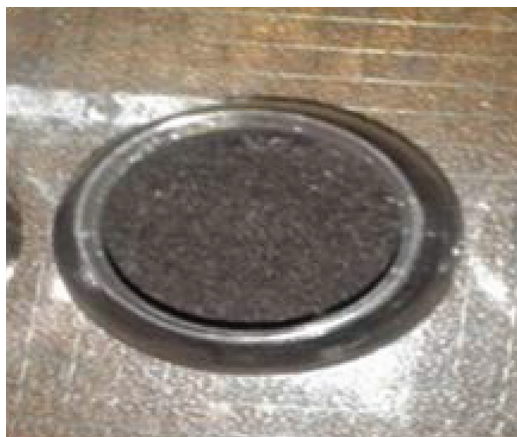
Figure 3. NaOH-activated sugarcane bagasse charcoal
