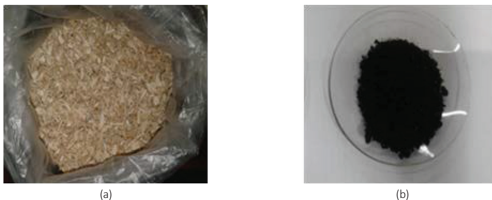
Figure 1. (a) raw sugarcane bagasse; (b) sugarcane bagasse charcoal
