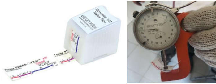
Fig. 5 Roughness measurement with Elcometer Testex Replica and Elcometer 124
