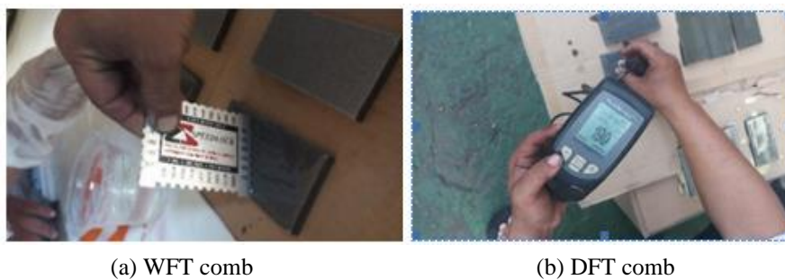
Fig. 7 Measurement of paint thickness
