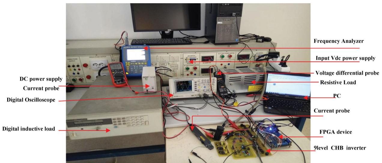
**Figure 13.** Photograph of the experimental prototype of the single-phase asymmetrical cascaded 9-level inverter.
