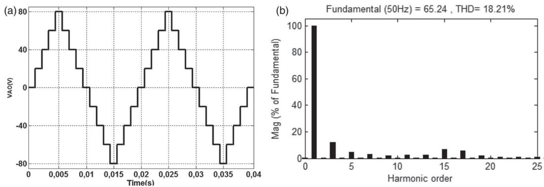
**Figure 9.** (a) Single-phase 9-level inverter output voltage waveform based on ESCA. (b) FFT analysis of the 9-level output voltage waveform (VAO) based on ESCA.
