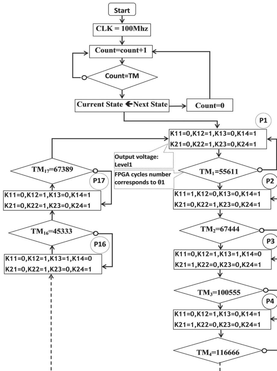
P<sub>i</sub> : represents inverter commutation cells states given in line i of table 4
