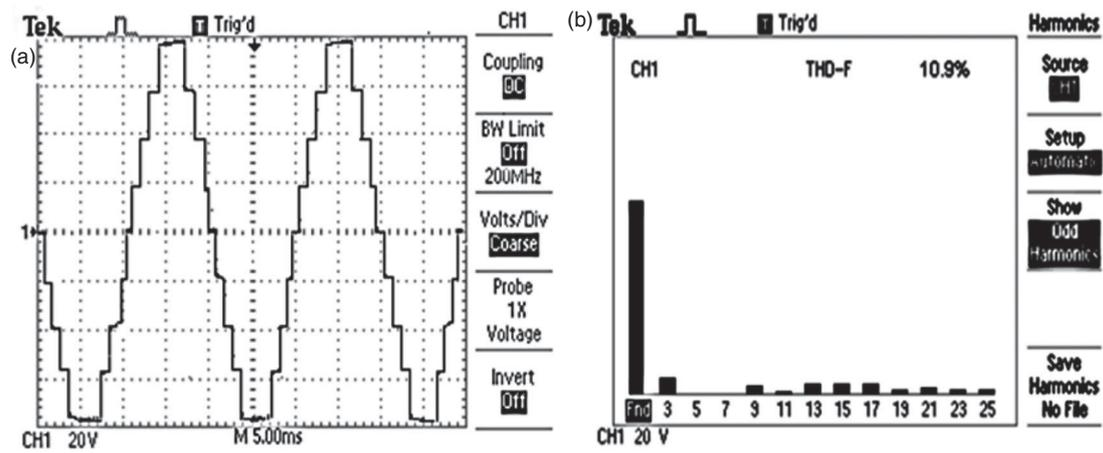
**Figure 15.** (a) Experimental result of the phase asymmetrical 9-level inverter output voltage based on N-R algorithm. (b) FFT analysis of the experimental 9-level inverter output voltage based on N-R.
