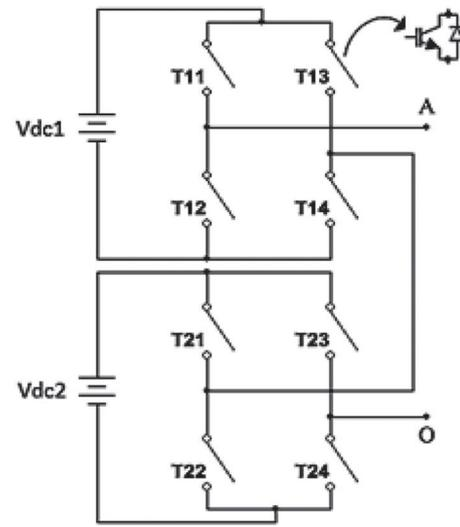
**Figure 1.** Single-phase topology of: (a) 5-level symmetric CHB inverter for  $V_{dc1} = V_{dc2}$ . (b) 7-level asymmetric CHB inverter for  $V_{dc2} = 2V_{dc1}$ , (ratio binary). (c) Asymmetrical 9-level CHB inverter for  $V_{dc2} = 3V_{dc1}$ , (ratio ternary).
