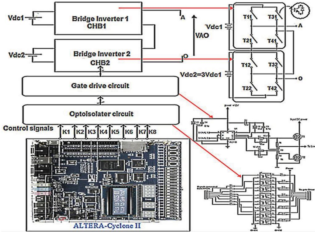
Figure 10. Block diagram of asymmetrical cascaded 9-level inverter using FPGA.
