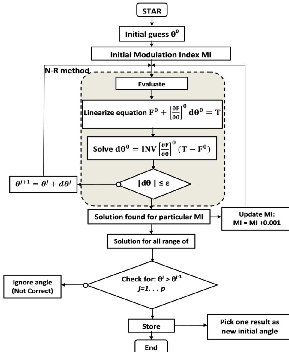
Figure 3. (a) Newton-Raphson flow chart of computer algorithm for solving the equation. (b) Genetic algorithm flowchart.
