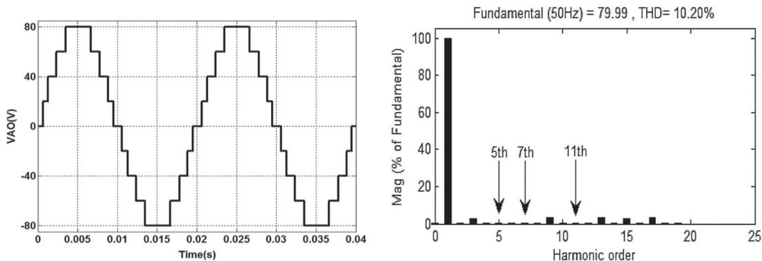
**Figure 7.** (a) Single-phase 9-level inverter output voltage wave form (VAO) based on N-R. (b) FFT analysis of the 9-level output voltage waveform (VAO) based on N-R Algorithm.
