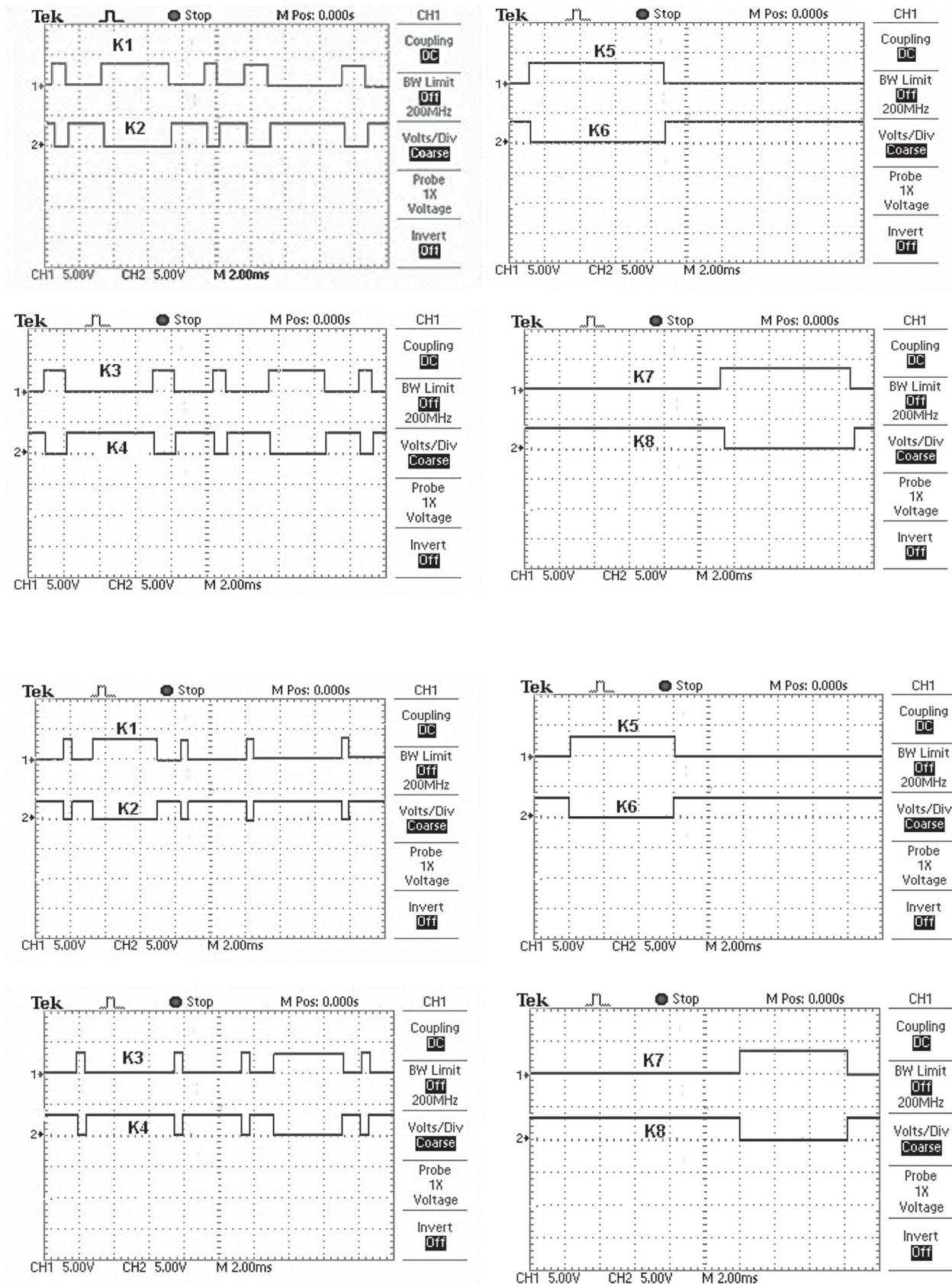
**Figure 14.** (a) Asymmetrical 9-level inverter control signals based on N-R generated by FPGA. (b) Asymmetrical 9-level inverter control signals based on G-A generated by FPGA. (c) Asymmetrical 9-level inverter control signals based on ECSA generated by FPGA.
