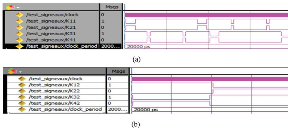
**Figure 12.** VHDL test bench simulation of the control signals for asymmetrical 9-level invert,  $r = 1$ : (a) HB1, (b) HB 2.
