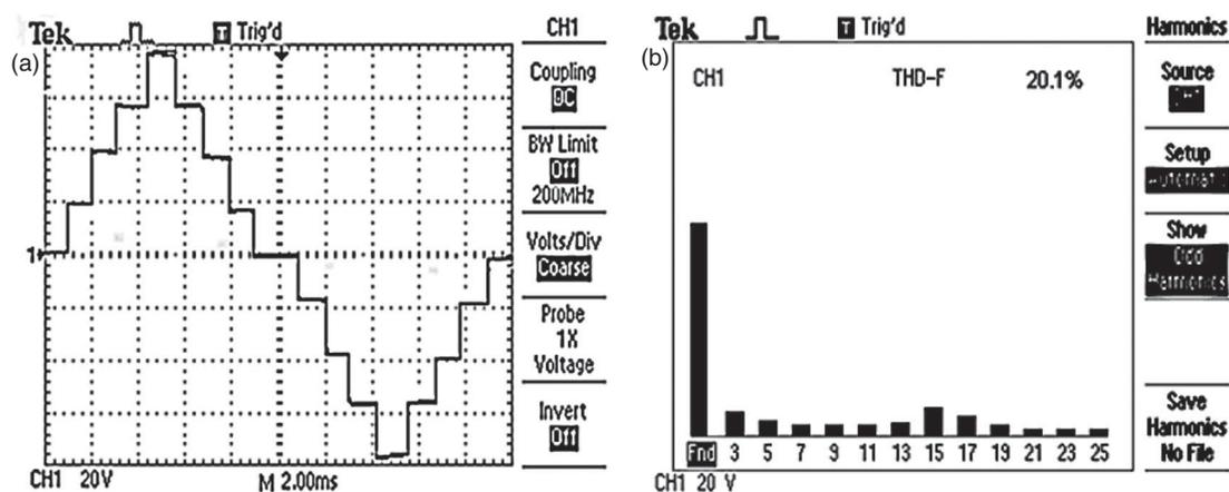
**Figure 17.** (a) Experimental result of the phase asymmetrical 9-level inverter output voltage based on ECSA algorithm. (b) FFT analysis of the experimental 9-level inverter output voltage based on ECSA.
