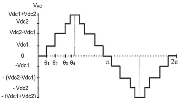
**Figure 2.** Staircase CHB 9-level inverter output voltage.
