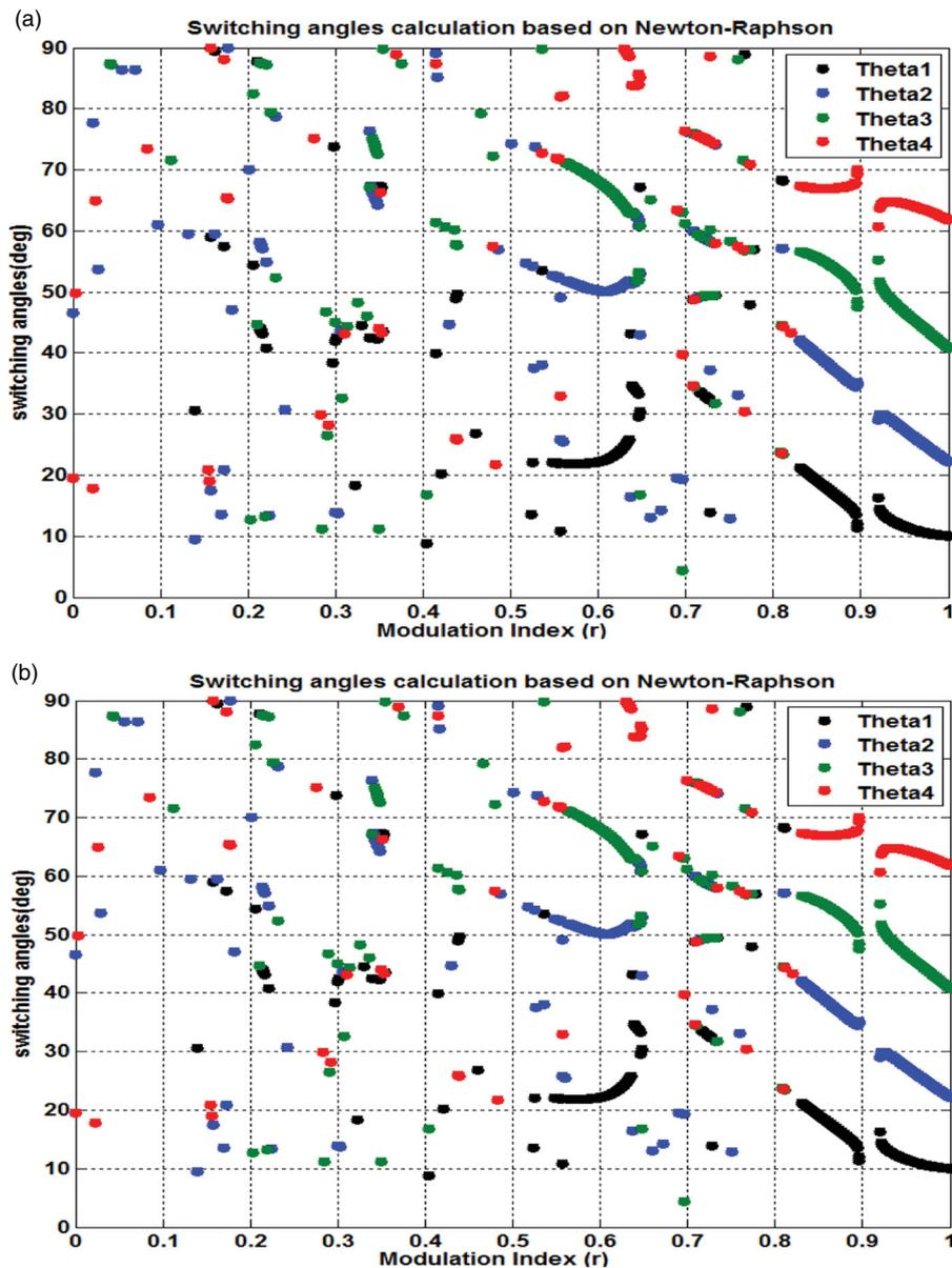
**Figure 4.** (a). Switching angles versus modulation index based on Newton-Raphson technique. (b). Switching angles versus modulation index based on Genetic Algorithm.
