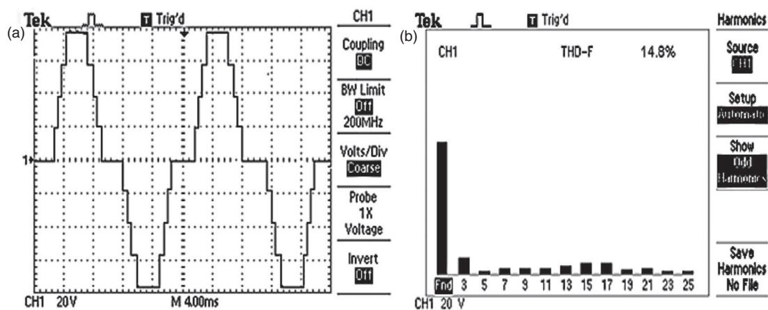
**Figure 16.** (a) Experimental result of the phase asymmetrical 9-level inverter output voltage based on GA. (b) FFT analysis of the experimental 9-level inverter output voltage based on GA.
