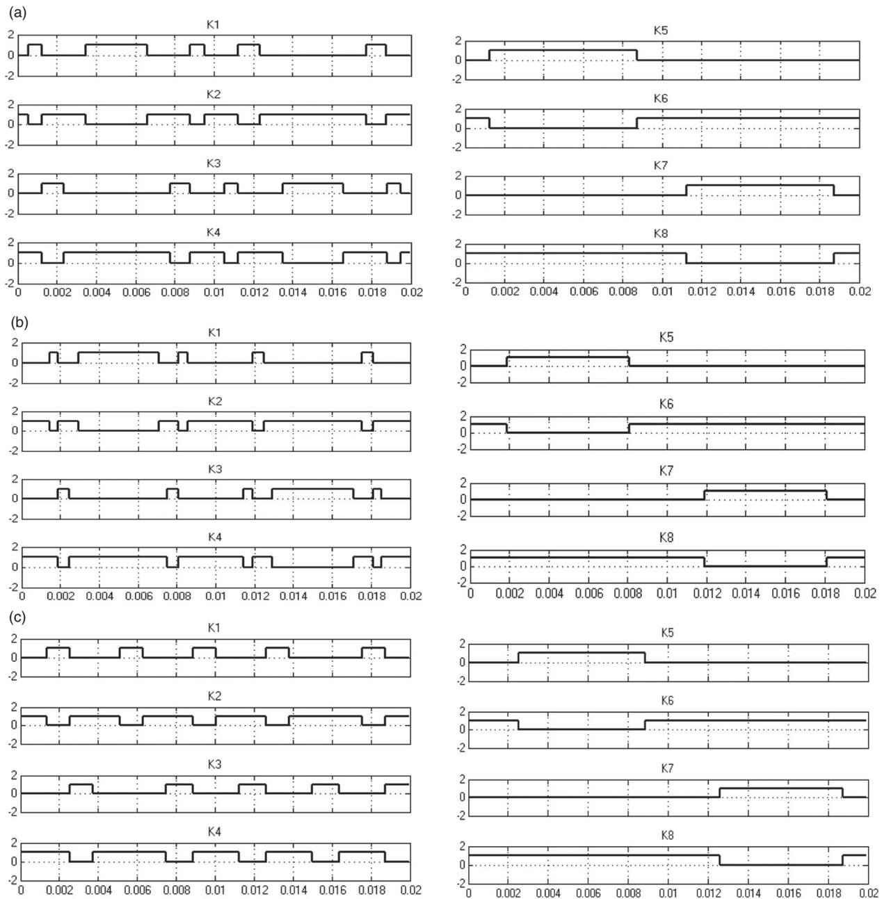
**Figure 5.** (a) Asymmetrical 9-level inverter control signals based on N-R. (b) Asymmetrical 9-level inverter control signals based on G-A. (c) Asymmetrical 9-level inverter control signals based on ECSA.
