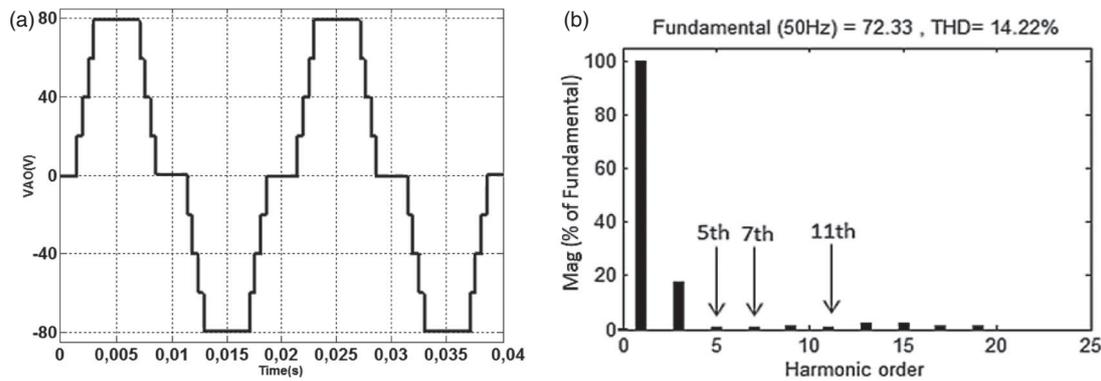
**Figure 8.** (a) Single-phase 9-level inverter output waveform based on G-A. (b) FFT analysis of the 9-level output voltage waveform (VAO) based on G-A.
