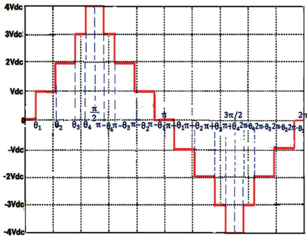
**Figure 6.** Inverter output voltage levels according to switching angles.
