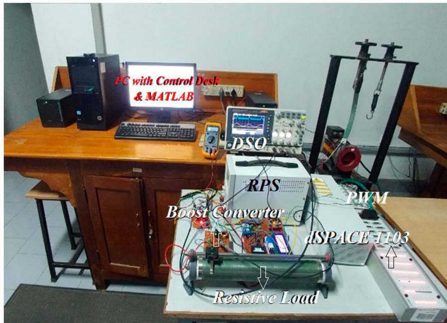
Figure 14. Experimental setup of the photovoltaic system.
