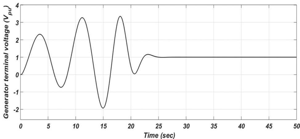
**Figure 11.** The voltage response of GES with  $K_p = 0.2, K_i = 0.2, \tau_2 = 1.5s$ .
