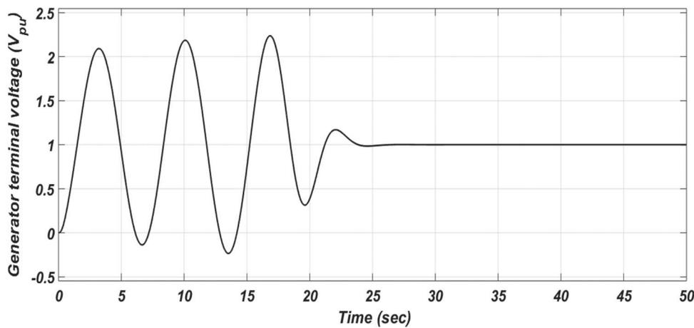
**Figure 10.** The voltage response of GES with  $K_p = 0.2, K_i = 0.2, \tau_2 = 1.2s$ .
