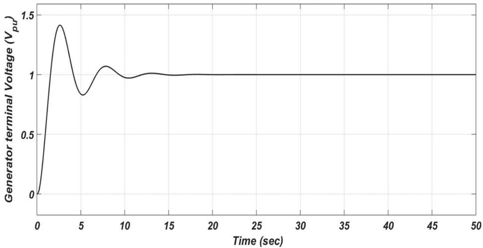
Figure 8. The voltage response of GES with  $K_p = 0.2$ ,  $K_i = 0.2$ ,  $\tau_2 = 0.5s$ .
