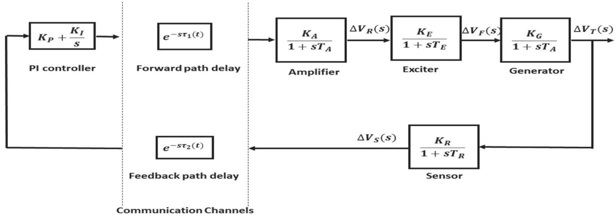
Figure 3. Block diagram of the GES
