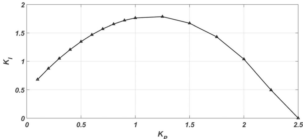
Figure 4. Controller capability curve for  $K_p$  vs  $K_i$ .
