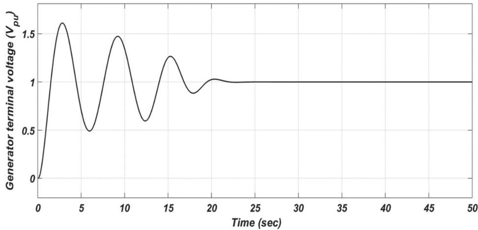
**Figure 9.** The voltage response of GES with  $K_p = 0.2, K_i = 0.2, \tau_2 = 1.0768s$ .
