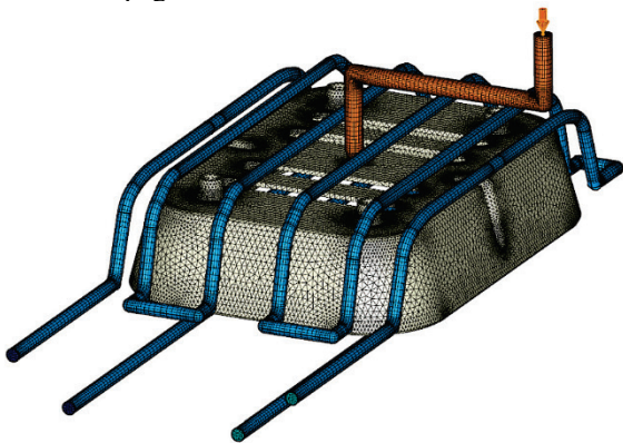
Figure 26 Simulation model with hot runner system and conformal cooling channels
