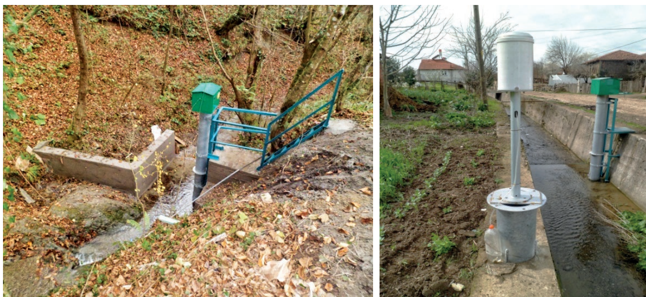
Figure 3. Streamflow gauging station installed in the FW (left) and the AW (right) Slika 3. Mjerna stanica vodotokova u FW (lijevo) i AW(desno)
