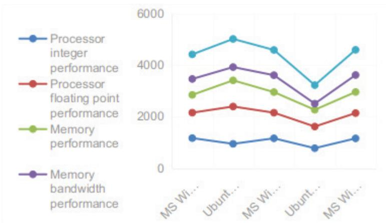
Below are the test results of the computer purchased in 2006. (B1, B2, B3, B4 & B5, 2014) Chart 2 shows that in this case the best results were achieved using the older version of the GNU / Linux Ubuntu 12.04 LTS operating system.
