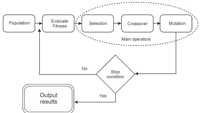
Fig. 1. Basic structure of a genetic algorithm.
