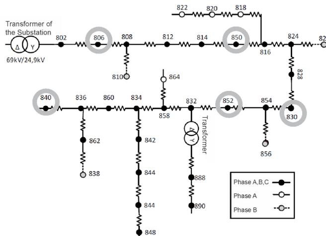
Fig. 7. Graphical representation of the bars selected in the optimization process 45 th-generation
