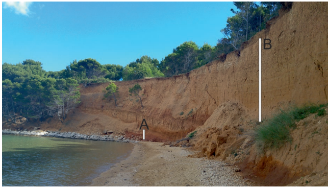
Figure 3. Outcrop of alluvial – aeolian sediment at the shoreline on Vrgada Island in the form of a coastal cliff. Sections A and B display the exact sampling locations. Note that the outcrop provides the mixed sandy-gravelly material for the approx. 8 m wide beach.
