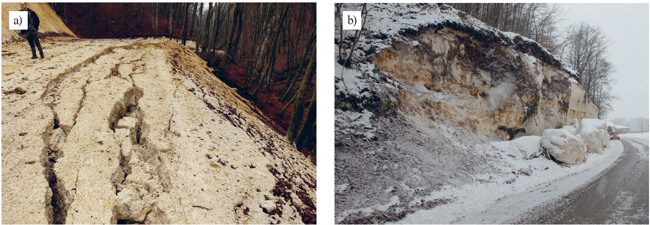
Figure 8. Coseismic landslide activation: a) slide in forest road embankment (near Strašnik, observation point ŠP-3); b) rockfall near Pecki that blocked the local road (observation point IK-ODR).
