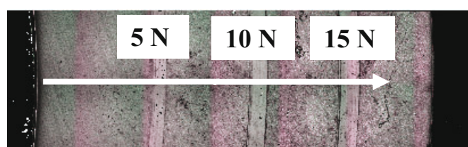
Fig. 3 The principle of measuring the magnitude of wear on the Alicona device
