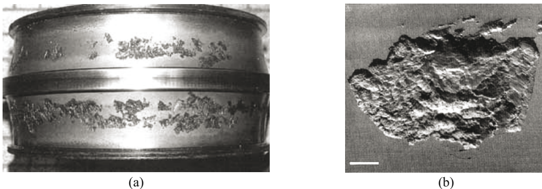
Fig. 1 Bearing ring wear caused by materials in contact: a) fatigue spalls on the outer bearing race, b) spall crater - detail [1]
