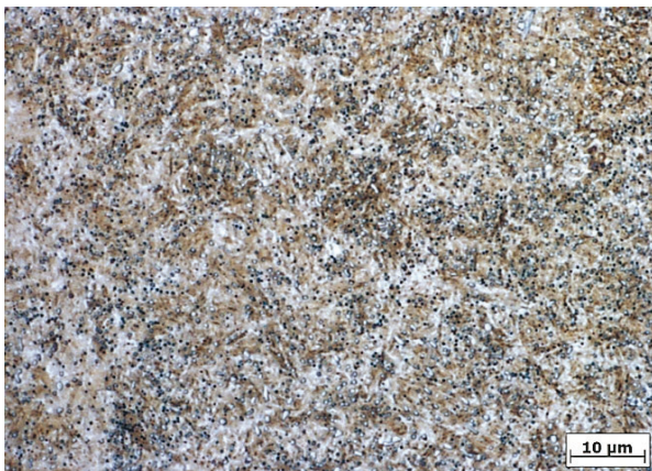
Fig. 4 Specimen microstructure: base material after heat treatment, etched in picric acid, optical microscopy
