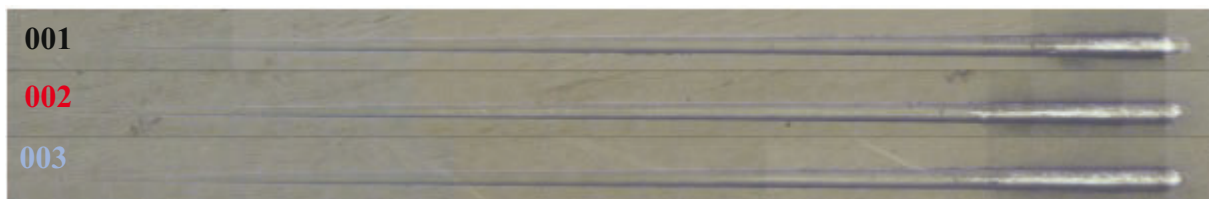
Fig. 12 Morphology of traces on the Sucaslide DLC coating after the scratch test
