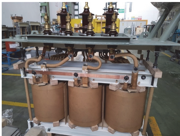
Figure 11 Active parts of prototype transformer
