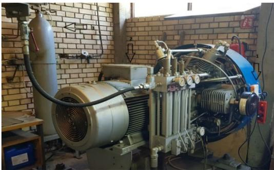
Figure 1 Compressor station type SVB 1300/359
