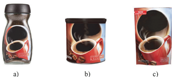
Figure 1 Test samples for coffee: a) glass, b) tin, c) flexible composite material
