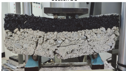
(d) Bending failure of specimens Figure 8 Bending failure of specimens
