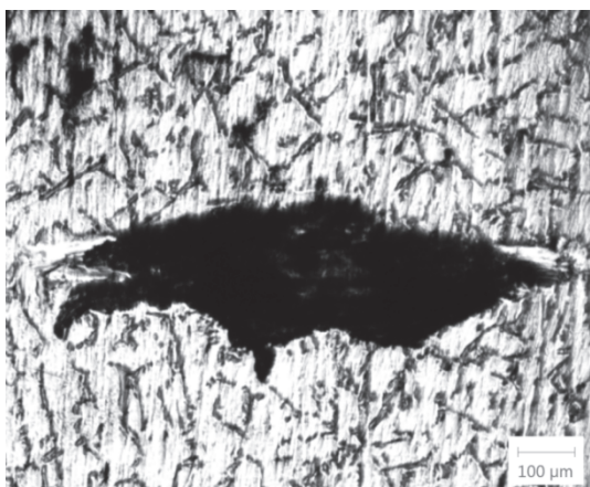
Figure 13 Surface micrograph of base material after dry sliding test under ( F_N = 0,6 \text{ N} , v = 9 \text{ mms}^{-1} )
