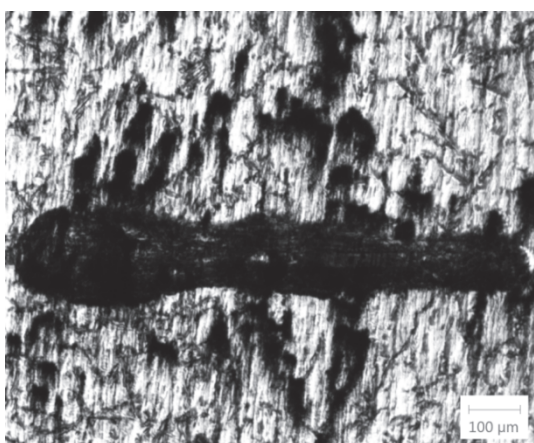
Figure 14 Surface micrograph of base material after dry sliding test under ( F_N = 0,6 \text{ N} , v = 15 \text{ mms}^{-1} )
