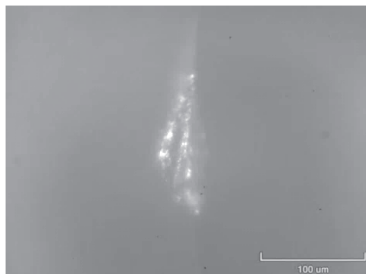
Figure 25 Optical microscopy of the counter body steel ball profile after sliding test against base cylinder material (Al alloy) (side view)
