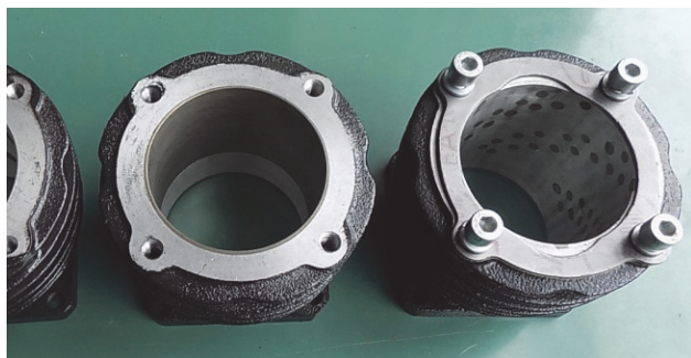
Figure 1 Photography of experimental cylinder samples. Left is cylinder coated with thermal spray method and right with reinforcements (nodules)
